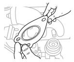
Position the turbo onto manifold or engine block using the correct new gasket or O ring, and then reconnect the exhaust pipe. Tighten all nuts and bolts.
