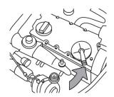
Clean the engine breather system (Positive Crankcase Ventilation system) and ensure that it functions properly.
