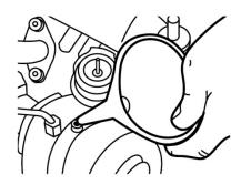
Pour new engine oil into the oil inlet hole of the turbocharger.
